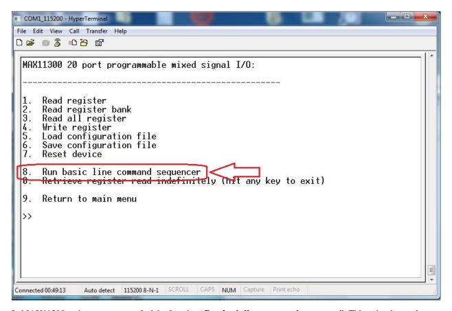
In MAX11300 main menu you can find the function "**Run basic line command sequencer**". This a simple *step by step* sequencer that performs READ and WRITE of Pixi register. It can be used to dynamically check basic input/output sequences and see on terminal the result of each step. It is possible to activate one or more *loop* to retry up to 65535 times any step group defined during line command insertion. By typing "8" in main menu screen, you go to sequencer sub-menu.
