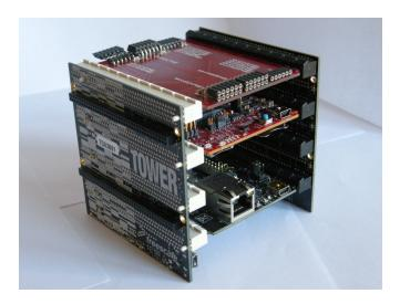
Don't care slot position, but be careful to connect Primary and Secondary connector properly. Take care at reference signed near PCI board connectors.
