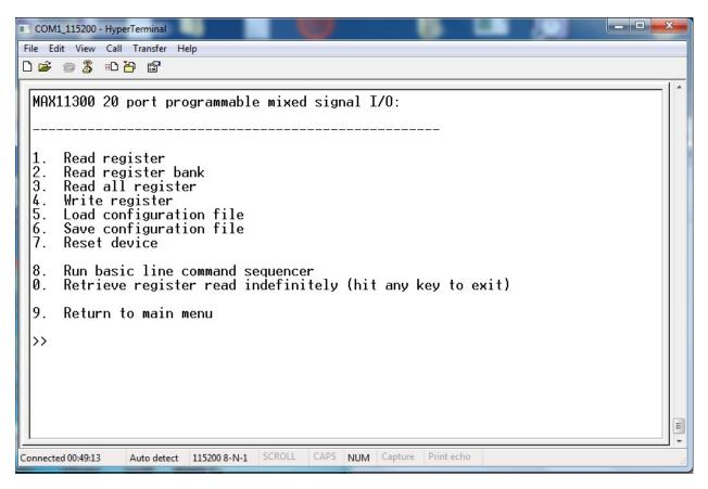
Follow instruction on screen to perform basic read/write functions or reset device to power-up default
