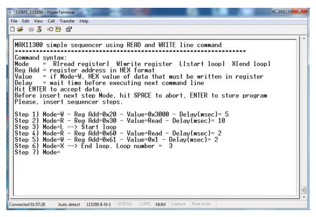
Read simple help lines to understand how to write command line. In the figure above you can see one program example. Data will be accepted when you hit ENTER. By typing ENTER when the sequencer editor will wait for MODE, the program will be ended and stored inside program memory.
