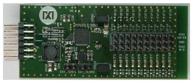
The new release v2 is able to evaluate MAX11300 PIXI, 20-Port Programmable Mixed-Signal I/O with 12-Bit ADC, 12-Bit DAC, Analog Switches, and GPIO. Full description of Pmod Pixi's functions loking at specific chapter. For installation and configuration you can use same intructions as you can find in chapter "Installing Codewarrior on WIN7 or WIN8" and "Quick Start Guide"
