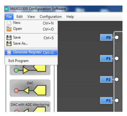
The MAXIM application will store a ".csv" file format, that can be read by Pmod1\_6\_v2 and stored inside the MAX113000PMB1 evaluation board.
