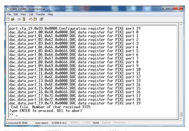
When transfer ends, press "ENTER" to start programming device, "DEL" to abort
