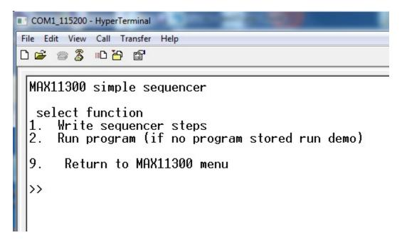
In the Sequencer sub-menu there are two functions: | Write sequencer steps (enter by typing 1) | Run program (enter by typing 2)
